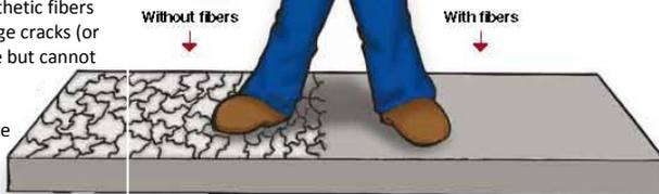
Synthetic macrofibers and steel fibers provide some bending strength and reduce crack widths but are not used as the only reinforcement in structural members like beams or columns. Macrofibers are longer (about 2 inches) and are added at higher dosages and don't bunch up during mixing.
