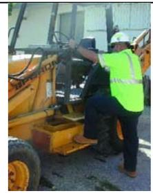
One of the most common causes of operator injury is slips and falls getting on and off equipment. Be sure to use a three-point stance when climbing into or exiting the machine.
