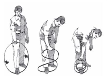
Folding a band saw blade is either an injury-defying task or a magic trick. It seems there are less band saws out there than there used to be, but for those who have band saws, folding a blade for storage is a must.
