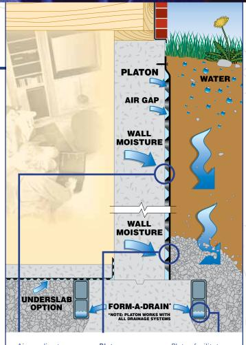
Air gap directs moisture evaporating from concrete walls out of your basement and into the drainage system.
