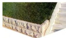
Corner blocks are used when you need to turn a 90° outside corner. It also can be used to simply create a texture face at the endof a wall to finish it off. Left and Right corner block are availble in both Standard and Top Block. The face of a corner block is 12" H x 24" wide, with a 12" return on the right side (right corner) or on the left side (left corner). Specify Right or Left and quantities needed when placing your order.
